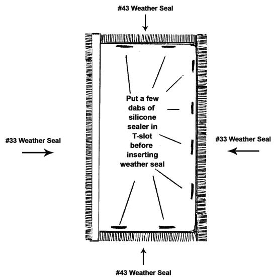
Put a few dabs of silicone sealer in T-slot before inserting the weather seal. We use Duro Clear Silicone Sealer. Make sure both sides of the backing are in the T-slots. Use the back edge of a blunt knife in the T-slot to get the plastic backing in the frame. Trim off the weather seal as needed to fit.
